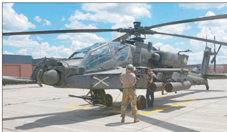
Electronics Mechanic Leader Jason Kilmer repairs the transponder on an AH-64D Apache Attack Helicopter at Fort Drum, New York.
